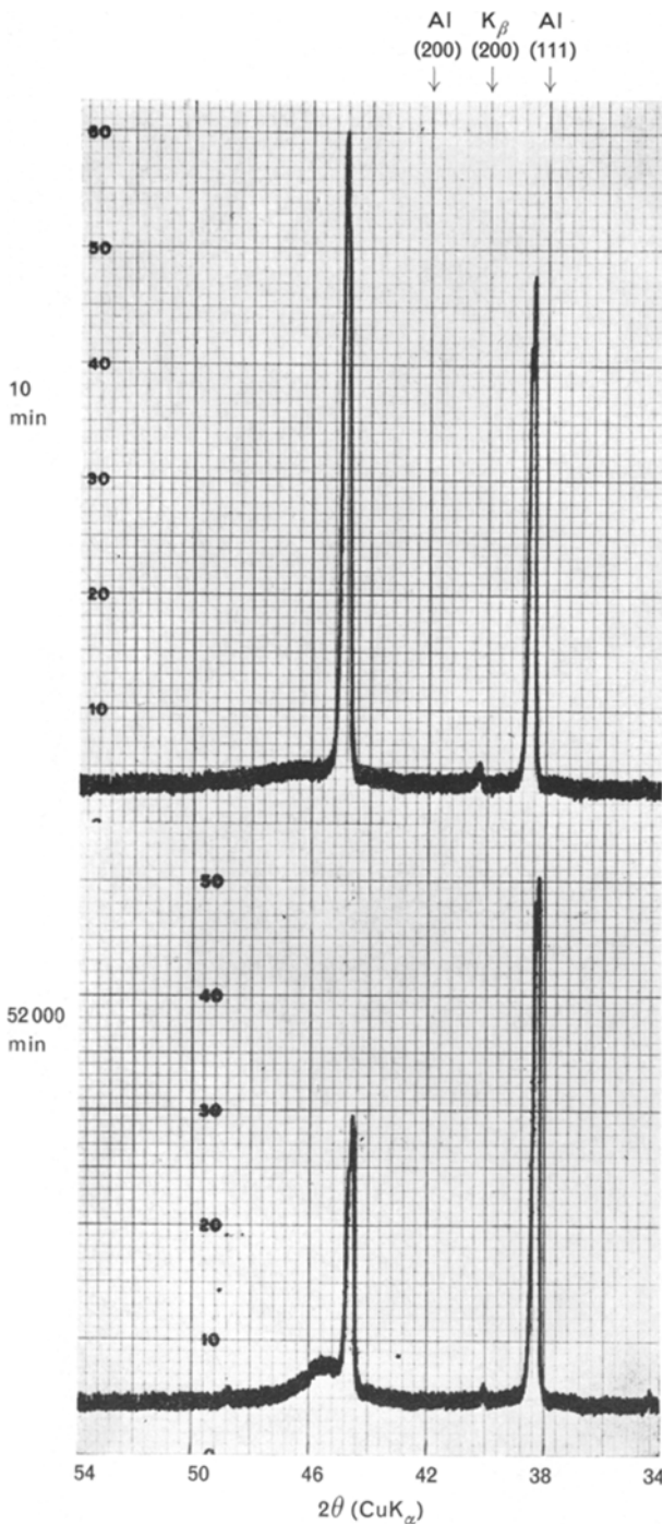
Figure 1 X-ray diffraction patterns of Al/38.5% Zn quenched from 365° C and aged at 22° C.
